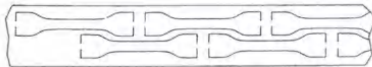
Figure 11 – Test pieces cut by grooved punch
